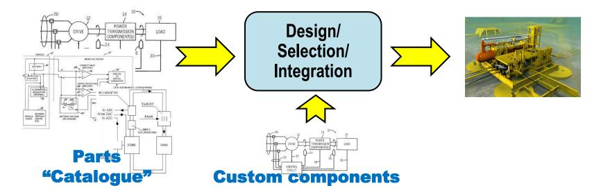
A particular system (product) is constructed by a <u>customer-specific configuration</u> of standard and custom components produced by the OEM and subcontractors
